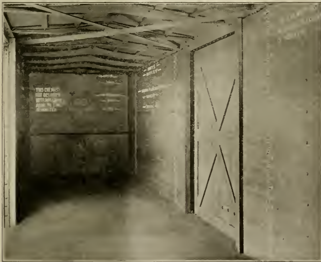
INTERIOR OF CAR, SHOWING HEIGHTS TO WHICH VARIOUS COMMODITIES MAY BE LOADED.
